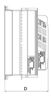
Control voltage (terminal A1, A2) = 230AC D = 234 Digital control voltage (terminal 1-5) = 24DC H = 388 Kg = 10.9 W = 175
